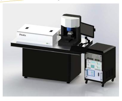
Sabray fs Micromachining System is a ultra-precision micromachining tools, which is mainly based on UpTek Solutions Corp's Phidia femtosecond laser system, Spearay series laser processing module, German Scoroff high-end cabinet, and with the features of compact structure. Sabray is proven for high reliability and stability in industrial grade long time application.
